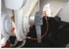
MECHANICAL LOCK FOR ALL OUTRIGGERS
