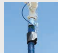
Shut Off valve on endhose
