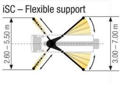
Dimensions can differ depending on configuration. Support width based on center of support leg. The specified values are reference forces.
